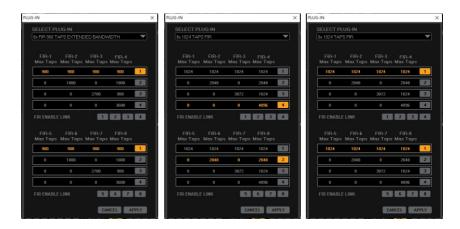
The output part, including gain, polarity, delay, IIR high and low pass filters, can be switched to MIR linear phase filter, or FIR filter can be used. Contains three dynamic processing modules: 8-band PEQ, RMS compressor, peak limiter, and hard limiter.
